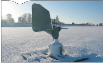
Figure 2. Volumetric spore trap (Burkard) in an experimental plot of wheat at INRA, Grignon, during the early winter phase of a septoria leaf blotch epidemic.
